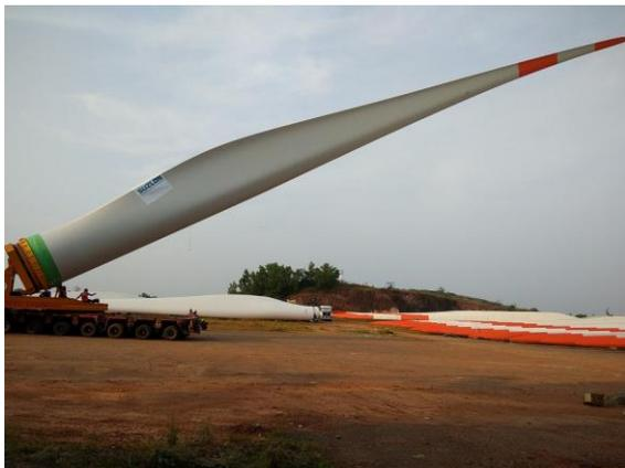
Suzlon SB63 blade mounted on an innovative adapter trailer
